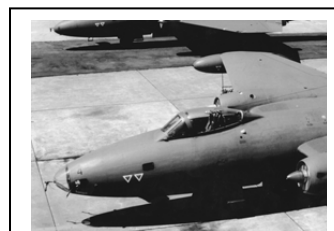
No ejection seat for the navigator despite the display of two ejection seat danger signs on the fuselage. (Paul du Bois)
