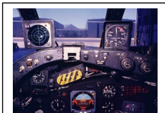
In the 1980's, the avionics were upgraded to include a new autopilot, a flight director and VOR/ILS which enabled flying coupled ILSs. (Pieter van Schalkwyk Collection)
