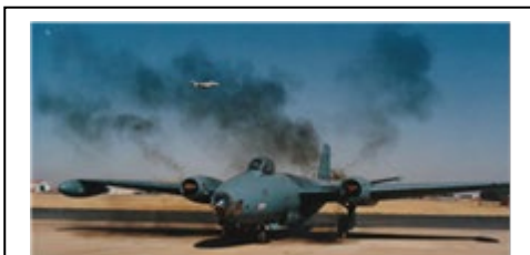
To any unsuspecting person near the aircraft, the ignition of the cartridge was announced with a very loud 'whoosh' as black smoke poured out of three cartridge exhausts – the engine start was something to behold. (12 Squadron SAAF)
